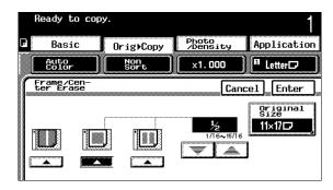
6 If the settings for frame-erasing or center- & frame-erasing are selected, touch and to specify the width of the area at the book edges to be erased. The width of the area erased with the center-erasing setting cannot be changed by touching and .
